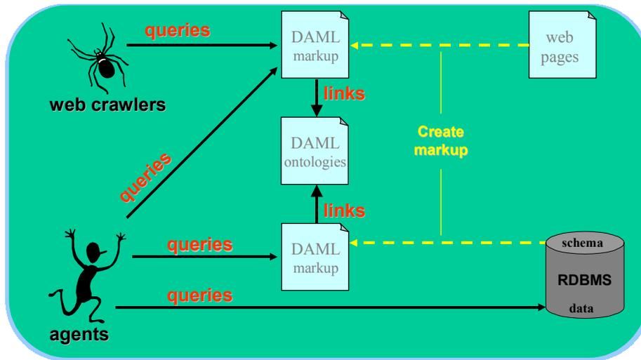
**Figure 1** – DAML markup for artifacts such as web pages, database schemas, legacy software interfaces, and sensor outputs.
