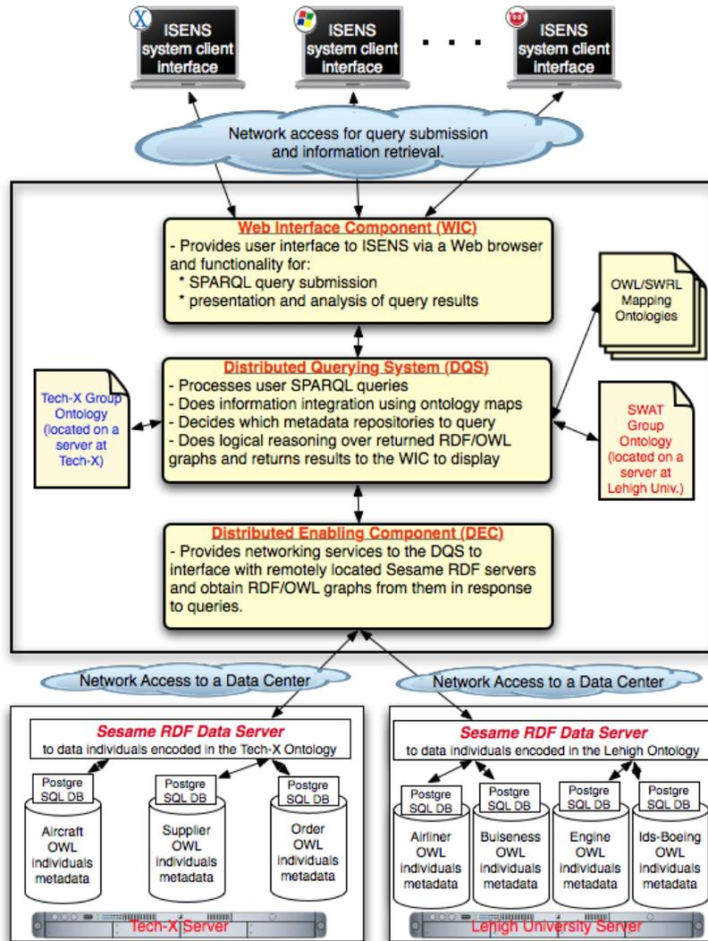
**Fig. 1.** The architecture of the ISENS prototype system is currently configured for querying of distributed RDF/OWL metadata at two data centers: one at Tech-X Corporation and the other at Lehigh University. The OWL individuals data is stored in multiple PostgreSQL databases that are managed by Sesame RDF servers. The Sesame servers provide remote access to the OWL individuals data. This set up allows testing of ISENS in a distributed and heterogeneous environment.
